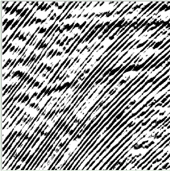
Figure 5. A noisy shot from the North Sea contaminated with steeply dipping noise of unknown origin.
